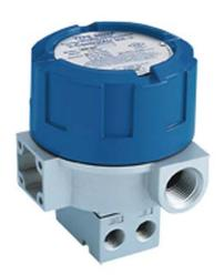
Control Air's compact T950XP I/P transducer delivers reliable high performance for the toughest applications in the most hazardous environments. The T950XP converts electical current signal to stable, pneumatic ouput to actuate valves. Advanced circuitry includes electronic feedback control for superior vibration protection and highly accurate output.
