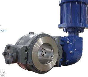
The 590's straight through unrestricted flow path provides higher capacity than globe style valves. A splined shaft provides accurate control in throttling operations and flexibility in actuation options. The 590 series, when combined with a Model DFRP piston actuator, is a rugged control valve assembly, to which a wide variety of positioners and accessories can be mounted.
