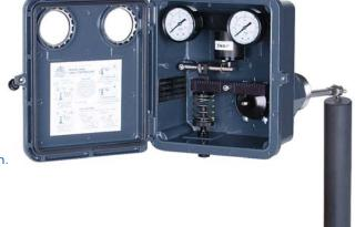
The 5000 level controller utilizes an innovative relay manifold design providing easy maintenance and improved safety. 5000 level controllers provide a pneumatic signal output for use with a control valve. The design of the 5000 allows for operational consistency through high and low pressure applications. 5000 level controllers are equipped with special access to the displacer arm seal, which can be serviced without disrupting the vessel connection.
